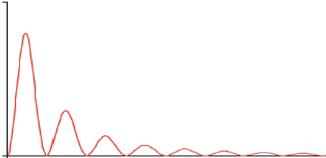
This function displays regular oscillations of constant period, with amplitude decreasing to zero.
